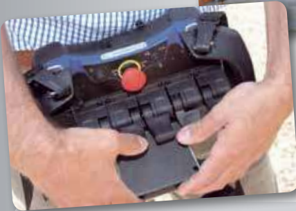
Remote control for all hydraulic functions
