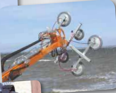
The Smartlift has hydraulic movements in all directions
