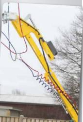
The beam has a manual extension in addition to the electrical.
