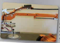
In addition to the electrical extension, the carrying arm is fitted with a manual extension arm to provide extra long reach.
