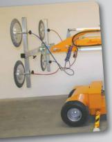
The vacuum system is separated into two vacuum circuits for highest security. Showing vacuum circuits with blue and red vacuum hoses
