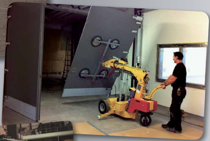
The SL 580 Maxi is increasingly used in industry for heavy lifting jobs.
