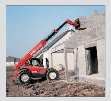
This carriage also enables you to use other equipment in the **MANITOU** range, such as the concrete skip with spout, and the fork extensions (1.70 m to 2.50 m).
