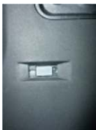
Fig. 7: Flight mode/panic switch
