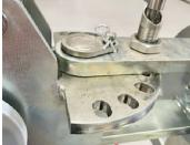
The vacuum head has two easy settings to allow for adjustment from canopy to table top lift
