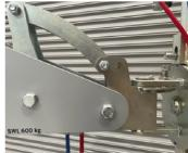
The vacuum head has 2 easy settings to allow for adjustment from canopy to table top lift
