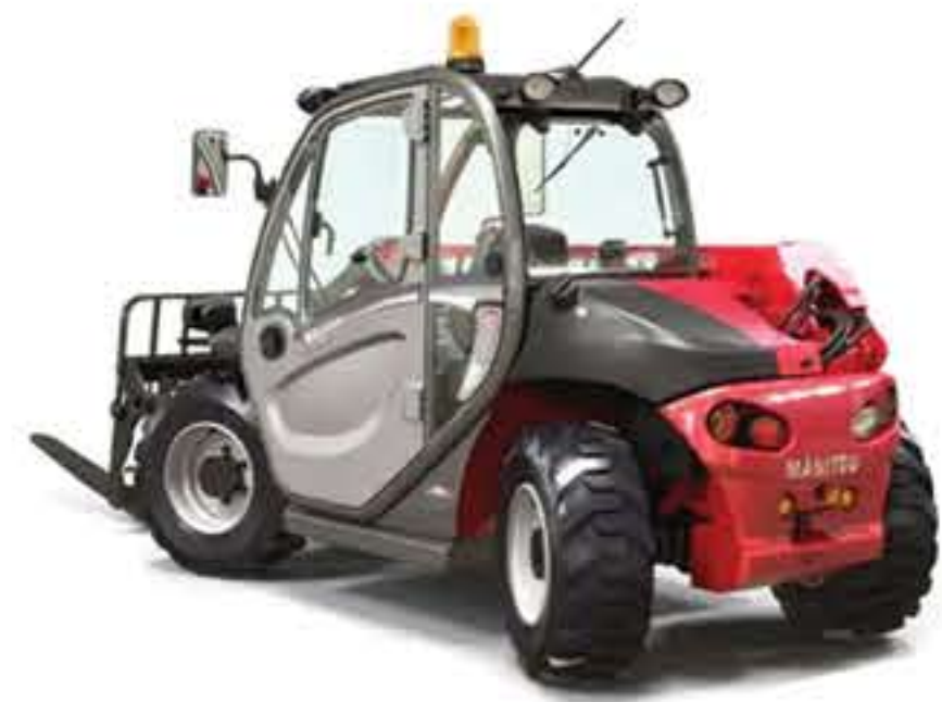
MT 420H COMPACT 2,000kg / 4.28m Small Turning Circle
